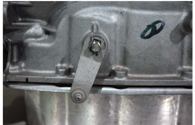
Figure 1: Install Shift Arm
