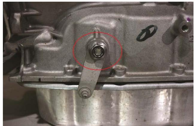
Figure 2: Install Shift Arm Nut
