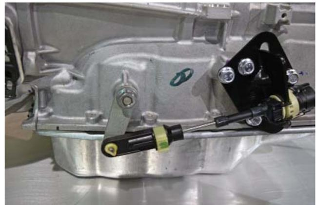
Figure 8: Install Cable End onto Shift Arm
