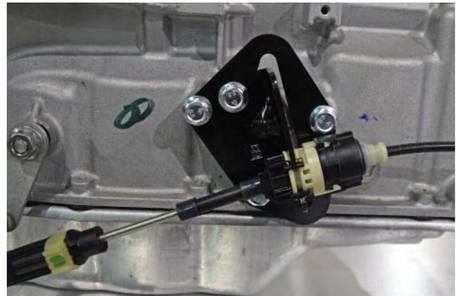
Figure 7: Install Cable to Bracket
