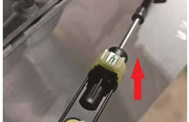
Figure 6: Release Cable End Adjustment
