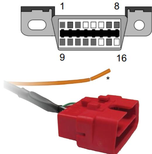
**\*NOTE:** The orange wire detects headlight status. If 12V is present on the green wire, display will dim for "Night Mode." This wire is only present on GDR series (round) indicators as GDS series (square) indicators automatically adjust to match ambient light levels.
